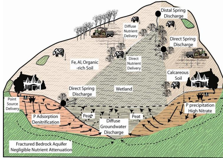
**Plate 1 (Left) :** Conceptual model of GWDEs in the Border Region. GWDEs receive groundwater through diffuse and/or point (spring) discharge. Nutrients applied in a catchment may leach to groundwater and to reach GWDEs. Groundwater flow regimes and geochemical conditions, particularly levels of **Ca**, **Fe** and **organic matter**, encountered along hydrological pathways influence the fate of nutrients, which may be removed by biological and chemical processes.
