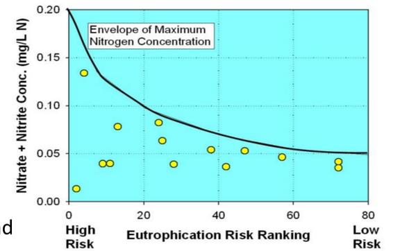
**Fig. 4 (above):** Plot of Nitrate plus nitrite concentrations in GWDE water samples for TIWEG field sites with risk ranking. Minimum concentrations differ little with risk, while maximum levels have a stronger relationship. This is suspected to reflect high levels of nutrient loss occurring in the subsurface.
